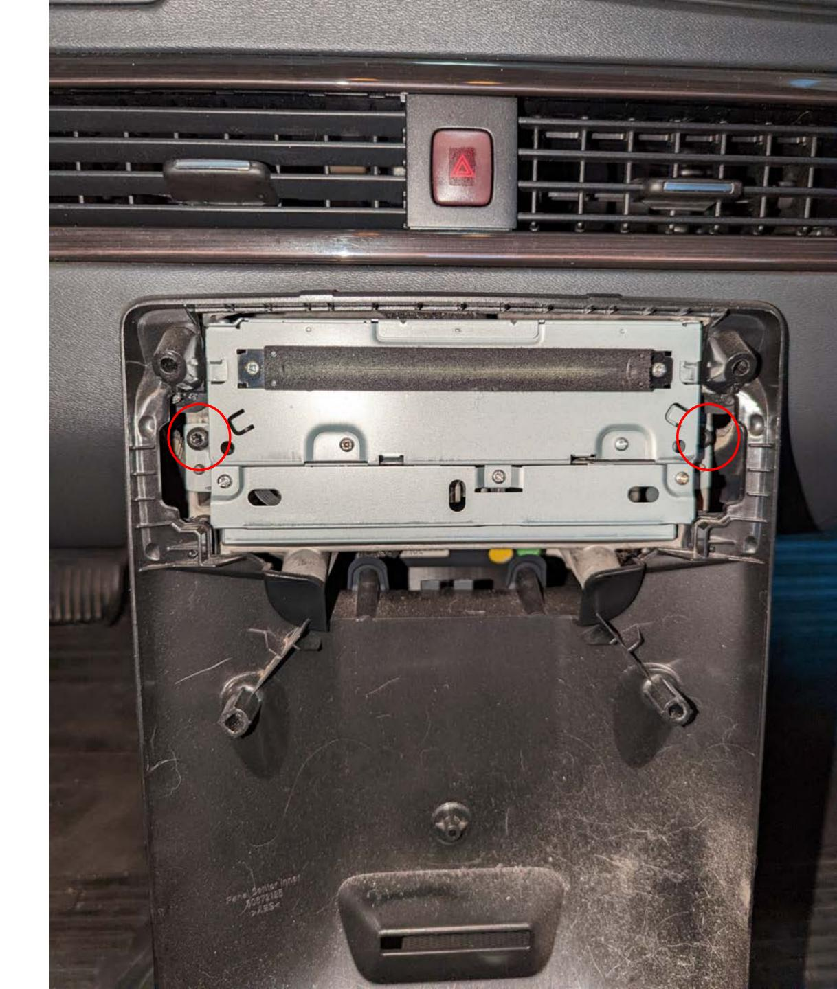
Pull the stereo out and loosen all of the connectors on the back of the stereo.
