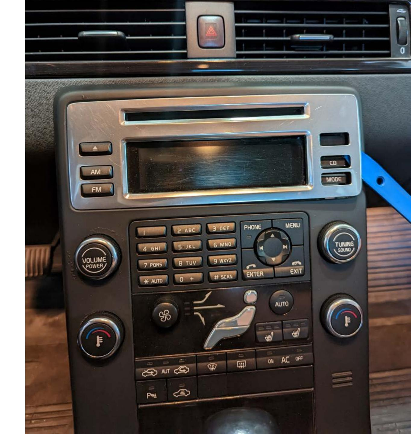
Use a plastic pry tool on the outer edge of the panel to pop it out.
